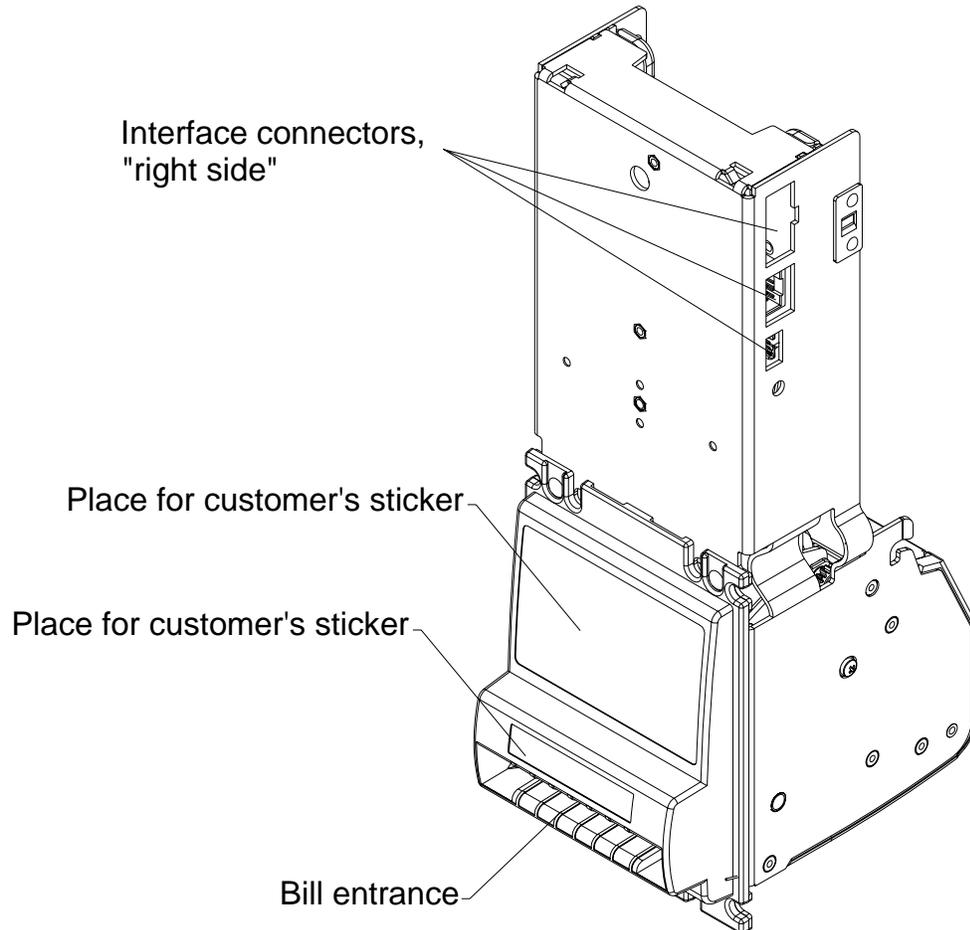
The MSM bill validator has all the required features that allow it to be used in any application.
