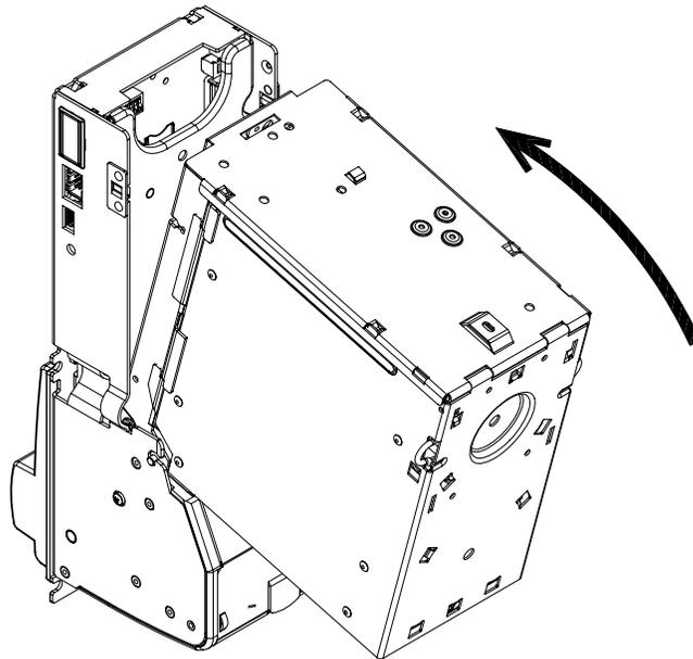
3. To remove the cassette, squeeze the two fasteners at the rear side of the cassette and pull the cassette. If the cassette carries additional locks, unlock them first.
