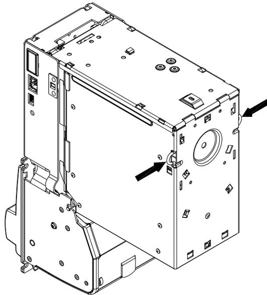
4. To collect bills from the cassette open the lock (or locks) at the cassette cover and open the cover. Remove bills. Close the cover.
