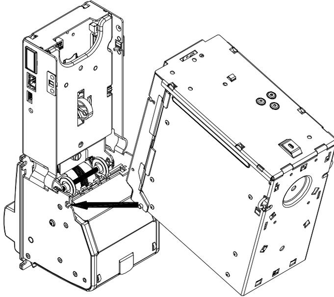
2. Rotate the cassette in the direction of arrow till fasteners of the cassette hook the latches at the validator housing. This action can be done for all types of cassettes whether they are equipped with second metal lock or not, as well as for the “gaming” cassette.
