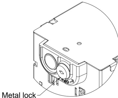
Every cassette can be equipped with the lock that locks the cassette to the bill validator. This optional locking mechanism is placed at the rear side of the cassette and prevents the removal of the cassette from the bill validator.
