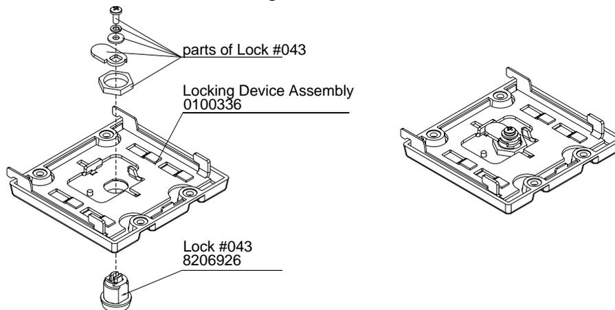
2. Insert the key into the lock and turn it to the “OPENED” position. Insert two tabs of the locking device into the slots in the cassette. Rotate the locking mechanism and insert two other tabs of the locking device into the corresponding slots in the cassette. Turn the key to the “LOCKED” position
