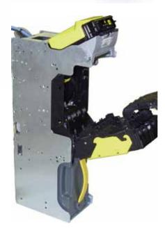
SCR is designed to ensure the entire note path is easily accessible for maintenance without breaching security protocol.
